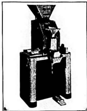
The unit weighs and fills bags, bottles, cartons, cans or envelopes. The mechanical action is unique in that the
